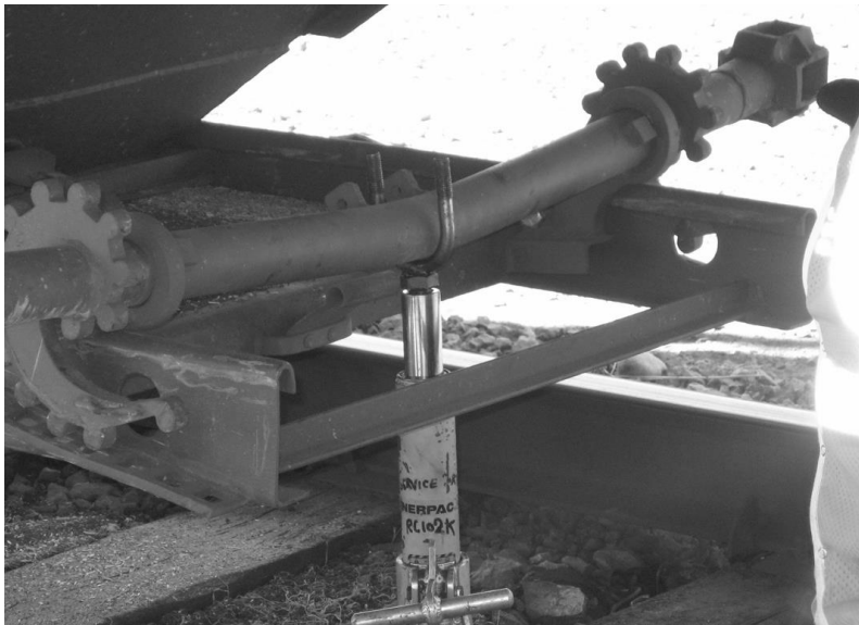
Bent hopper gate being repaired
