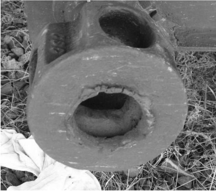
Damaged capstan (rounded square drive socket)
